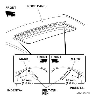
4. Using isopropyl alcohol on a shop towel, clean the roof area and the inside edge of the moonroof opening. Starting at the mark you made, clean about 2 inches toward the front of the opening but don't wipe off the mark.
