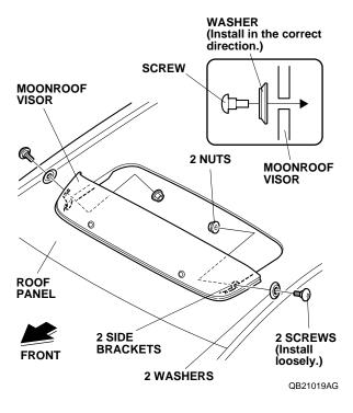
16. Position the moonroof visor with equal spacing in the front and on the sides. Check that the rubber molding is not twisted or rolled under the visor.
